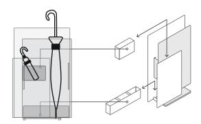
The SOU includes two removable containers to pick up the water. The smaller one it's located behind the front panel halfway up so the little umbrellas are accessible. The bigger container is located in the lower-inner part of the hind panel so the bigger umbrellas can fit well.
